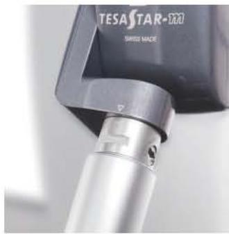
TESASTAR-m and TESASTAR-sm are motorized indexable probe heads, capable of indexing in 5° increments. This translates to a total of 2.952 positions in the measuring volume. These probe heads also feature high speed indexing - faster than similar products. The version TESASTAR-sm can be mounted inside the Z-ram of the CMM.
