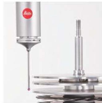
LSP-X1 is a highly accurate 3D scanning probe and compatible with indexable probe heads such as the TESASTAR-m. The probe offers both Single Point Probing and Continuous Scanning. There are different versions available suitable for various stylus lengths.
