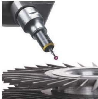
TESASTAR-p and TESASTAR-mp are compact 5-way touch-trigger probes. You can choose from four trigger forces: low, standard, medium or extended force. TESASTAR-mp consists of two parts: the sensor body and the stylus holding module. The modules can be quickly changed in manual or automatic mode through a highly accurate and repeatable magnetic isostatic clamping system – without the need for requalification.
