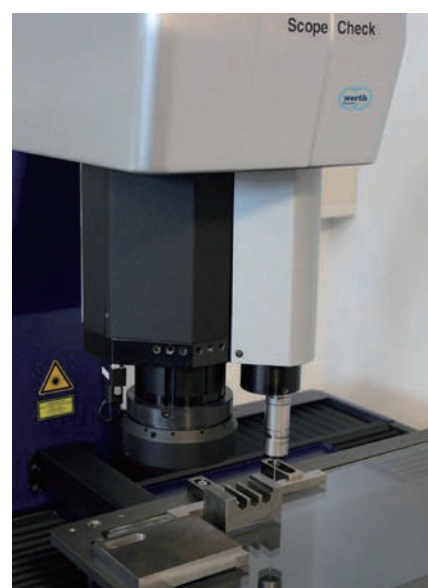
For tactile measurements, the components must be properly clamped to prevent them from moving. The fixtures are later used for process control in production
