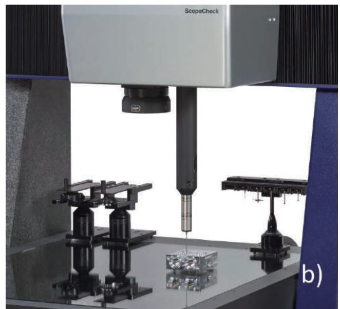
ScopeCheck® FB DZ with two independent sensor axes for collision-free measurement in the production environment: a) image processing sensor in use; b) scanning probe in use – the changing racks for the multisensor systems and the probe styli are in the background
