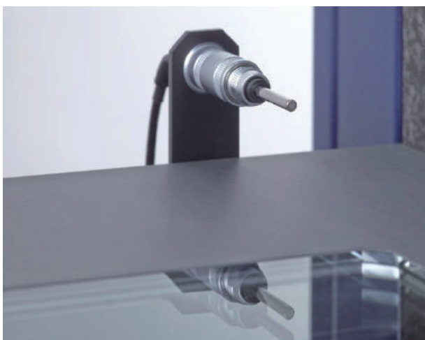
Temperature sensor in the measurement range
